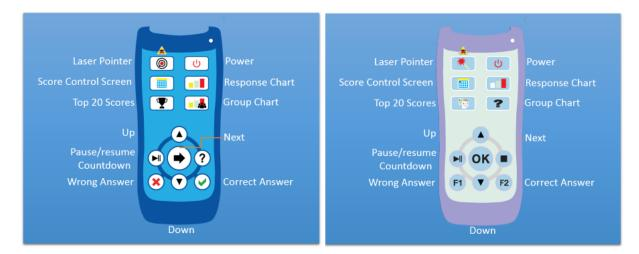
There are two versions of the remote control. A further explanation of the buttons can be found in the table below.
